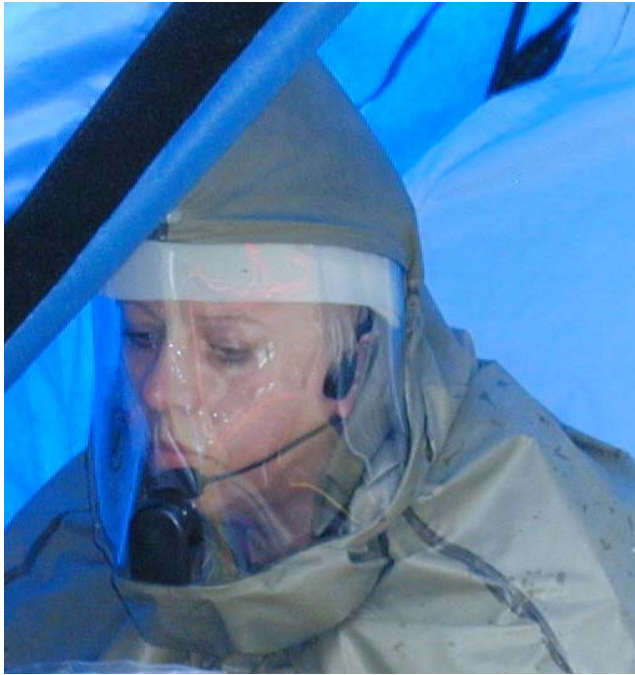
“Temple-transducer” style two-way radio headset stays in place under PAPER hoods.
